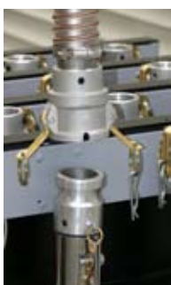
Attachment of a virtually indestructible RFID transponder on the coupling.
